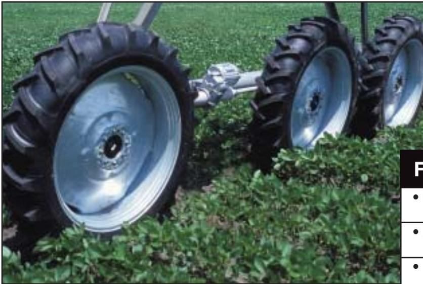
In challenging soil conditions, the V-3 drive unit will add the extra traction required to move through the field. It provides 50% more flotation than a standard drive unit to help get through rough spots and reduce rutting.
