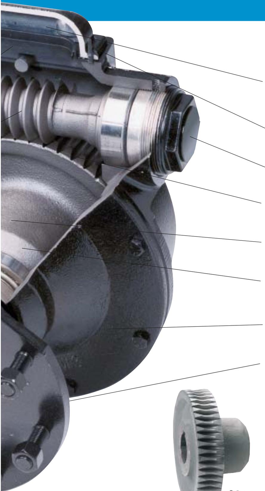
**Expansion chamber** — cap made of noncorrosive cast aluminum; rubber diaphragm allows oil to expand and contract during operation, minimizing pressure change to minimize water condensation.
